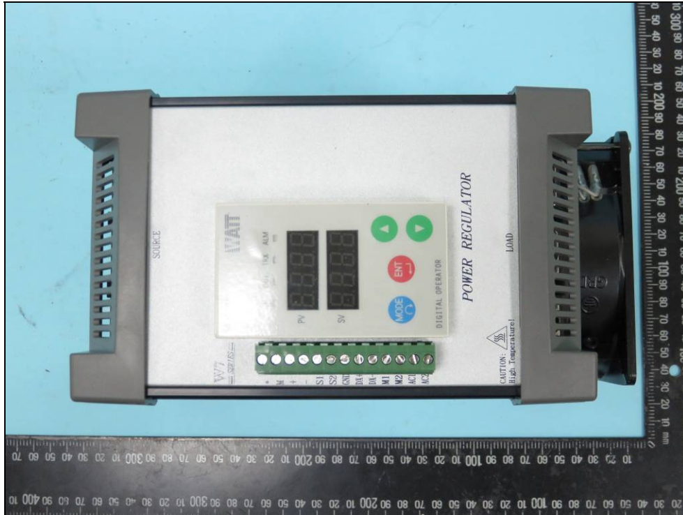
E.U.T. THYRISTOR POWER REGULATOR, Model W7T4V060-21KF
